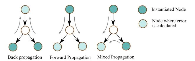
Estimating a hidden node is an optimisation process, and as a consequence runs the risk of being trapped in a secondary minimum. Therefore it is usually desirable to include some form of simulating annealing and to use a fairly slow step size. Alternating the different propagation methods can benefit the process since they do not necessarily adjust the parameters in the same way.
