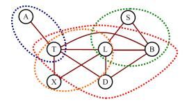
Grouping the nodes in cliques gives us four sets as follows: [AT], [SLB], [TLBD], [TLX]. We now need to define the running intersection property. This means joining the cliques such that for any clique those variables which appear higher up in the tree appear in its immediate parent node. We can do this by breadth first search starting from a clique containing a root of the original network. There is no unique solution, here is one ordering:
