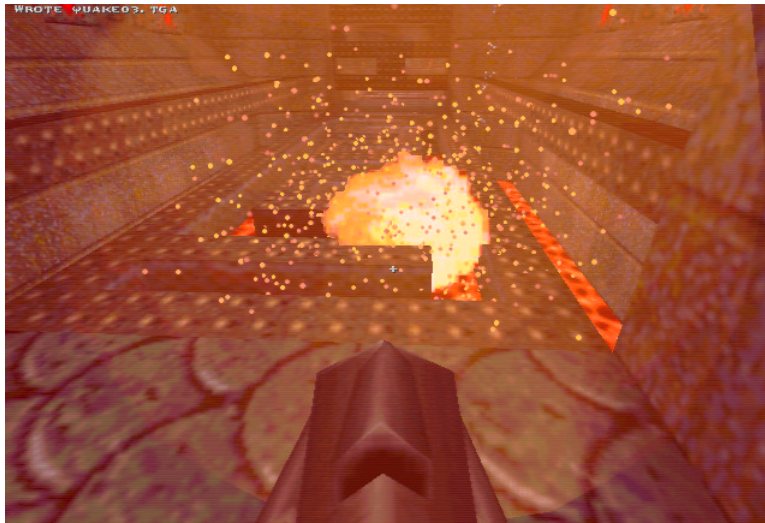
Figure 1.4: An example of fire from the computer game Quake [Carmack et al., 1996]. Notice that it is a hybrid of three components: 1) prerendered bitmap fire (the core), 2) a real time rendered glow (transparent spheres) and 3) the real time animated and rendered, glowing particles. The explosions work very well while playing the game, this snapshot, however, is another story. †
