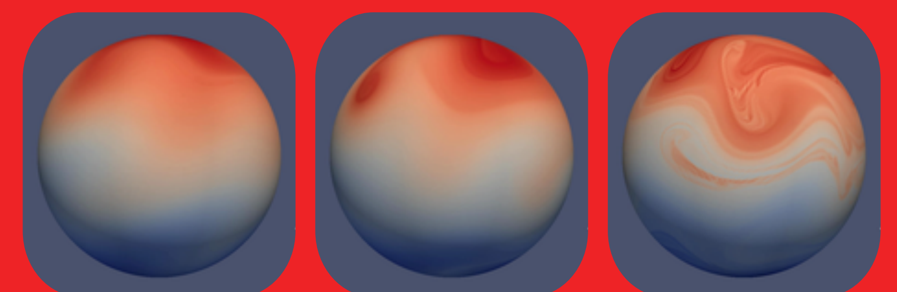
The evolving potential vorticity field in an idealised atmosphere simulation.
