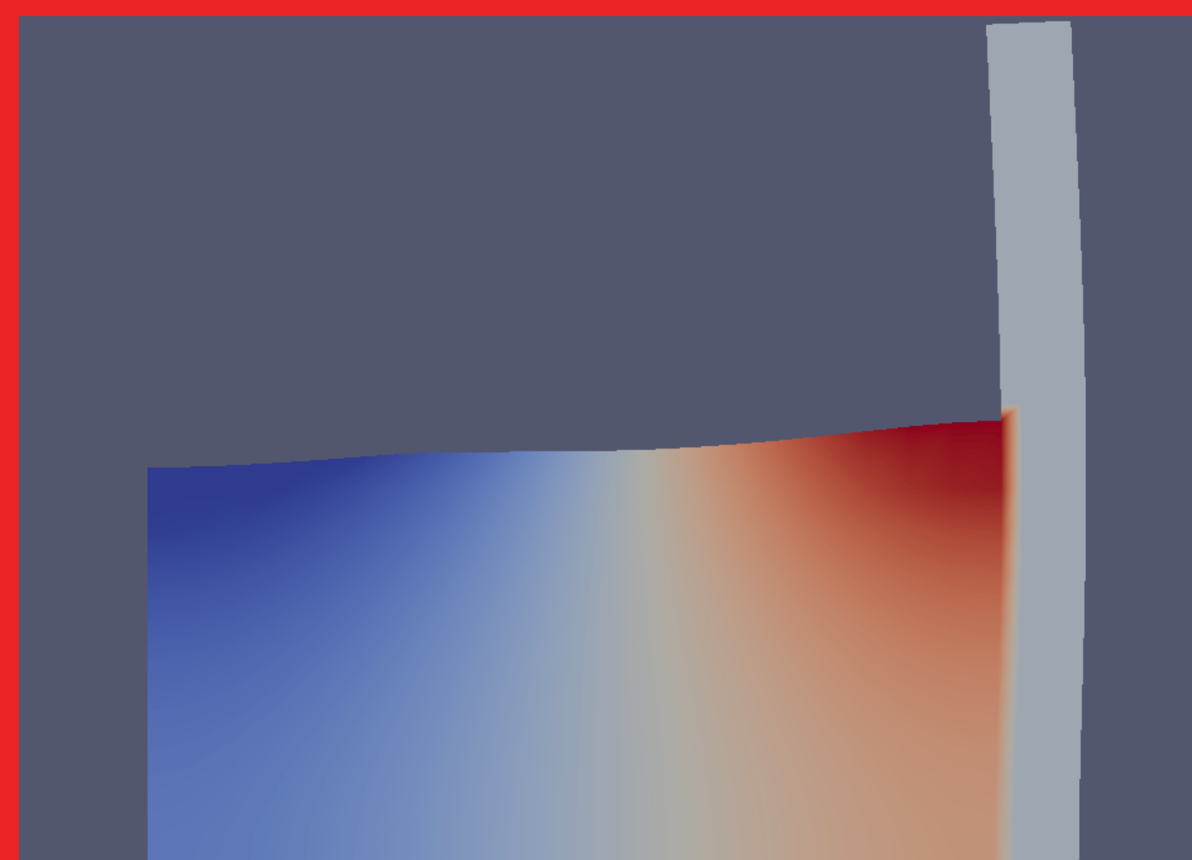
2D potential-flow fluid with a free surface (left) interacting with a monopile elastic solid (right).
