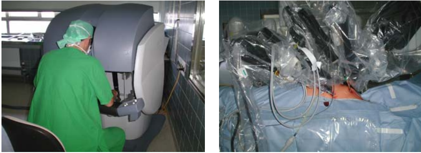
Fig. 1. A telemanipulator based system for minimally invasive surgery ( daVinci , Intuitive Surgical): The surgeon controls the instruments from a console that is providing a stereoscopic view on the operation area (left). The instruments and the endoscope are attached to the arms of the system, and inserted into the patient via ports (right)
