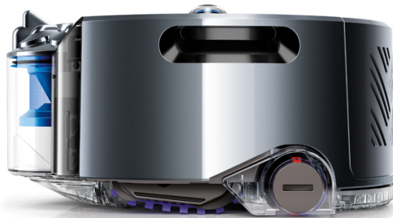
Figure 1.4: The Dyson 360 Eye. The vision sensor is visible at the top of the robot, a mirror which reflects the room into an upward facing camera.
