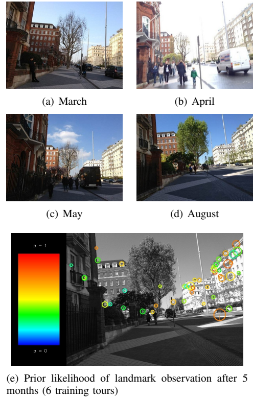
Fig. 2. The likelihood of a landmark being observed in a scene is calculated across all available training tours. Dynamic landmarks, such as those caused by moving bodies or tree growth, have a low likelihood, whereas strong structural landmarks, such as those caused by windows, have a high likelihood.
