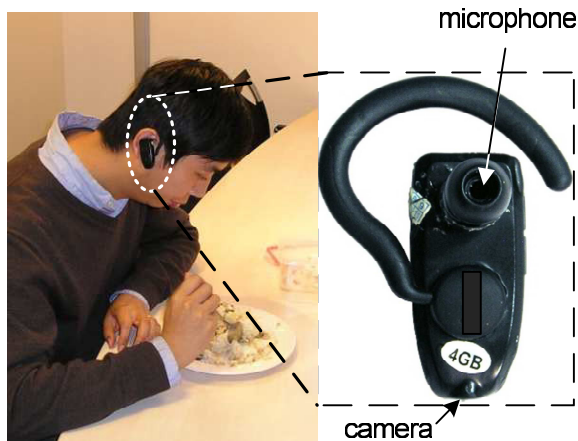
Fig. 1: Left: a subject wearing the food-intake sensor during lunch. Right: the profile of the sensor.
