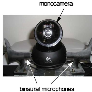
Fig. 1. Mobile robot head with binaural microphones and a monocamera.
