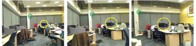
Fig. 5. SURF features detected in training images are tracked across other images in the database to form a set of landmarks. Here, all features representing the same landmark are assigned the same color.
