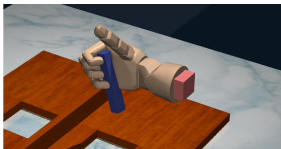
Figure 4.22: the stick slipping out from the MPL
