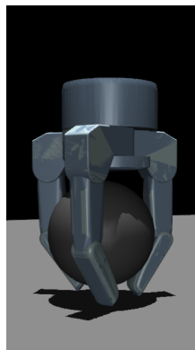
Figure 4.24: the Barrett hand in MuJoCo grasping a sphere with the output from GraspIt!
