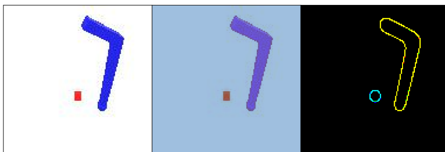
Figure 3.3: An image of 3DOF arm in various domains. Left: Original. Center: Tinted image by multiplying the colour channels by [0.25, 0.5, 0.75] respectively after pre-processing to values between a range of [-1, 1]. Right: Image created by putting each colour channel through a canny edge detector and recombining the colour channels.
