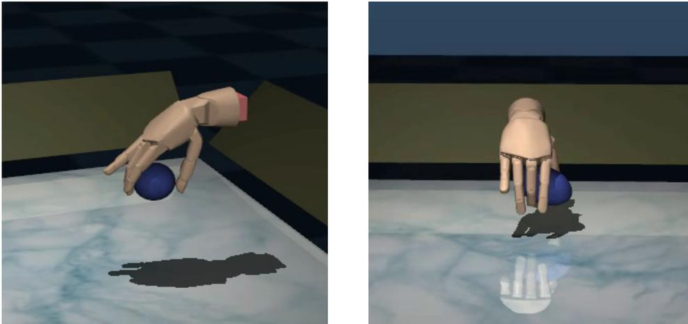
**Figure 6.21:** Objects intended to be grasped by three fingers were grasped by two fingers instead fingers were touching the object with their distal phalanx. From this we can conclude that more or larger touch sensors could have improved the results.
