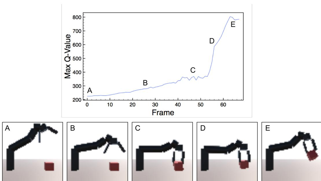
FIGURE 6.6: A frame-by-frame Q-value visualisation of a successful completion of a task. At each point in the episode, the highest Q-value is chosen and plotted. The labels from A to E correspond to the frame numbers in the graph.
