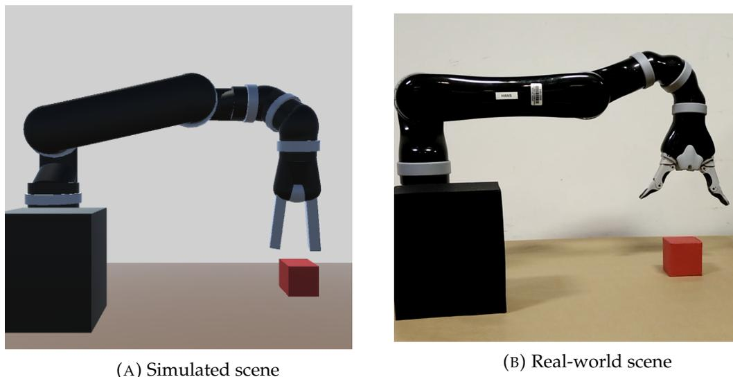
FIGURE 6.21: Preparing both the virtual and real-world scenes for training. A black box in front of the base in both scenes in order to avoid modelling the clamp holding the arm to the table.
