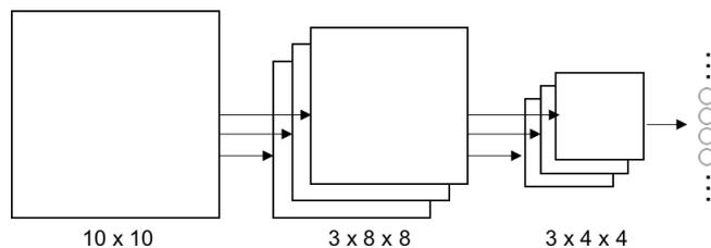
FIGURE 2.14: Convolutional layer, followed by a max pooling layer, and finally a fully connected layer.
