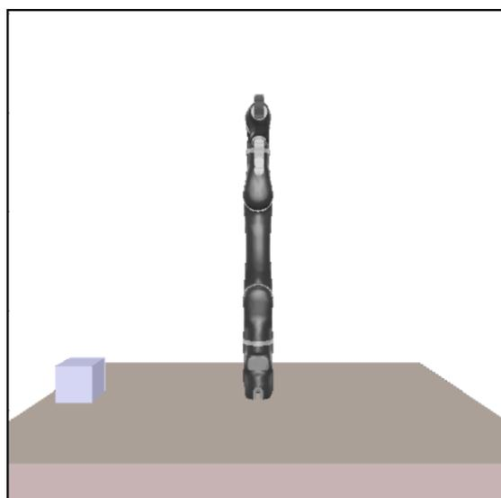
FIGURE 5.3: The starting position of our first experiment. Joint angles are set so that the arm is set in this position at the start of each episode.
