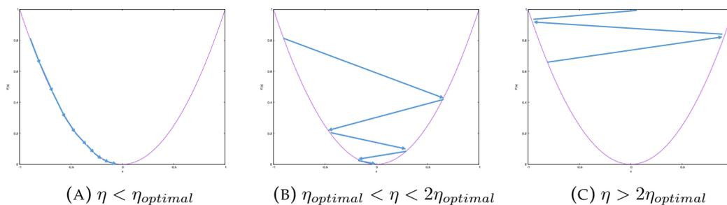
FIGURE 2.9: The effect learning rate ( $\eta$ ) has on convergence — where  $\eta_{optimal}$  is the value of  $\eta$  that would result in reaching the minimum in one step.
