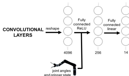
FIGURE 6.7: Concatenating the 6 joint angles and gripper state to the first fully connected layer of the network.
