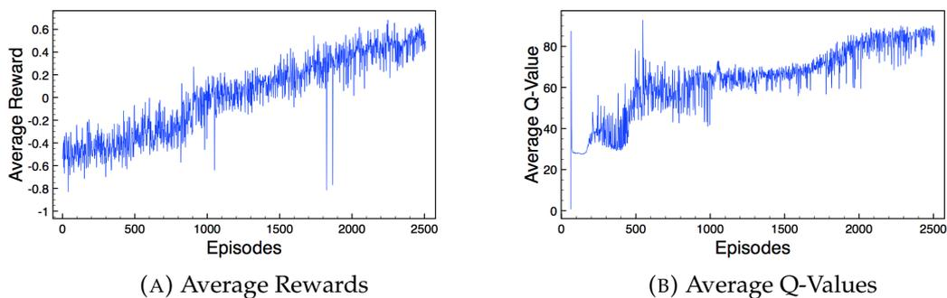
FIGURE 5.7: Results of using intermediate reward to guide the agent to pick up the cube. The agent did not succeed in picking up the cube once during training. Despite this, evidence of learning can be seen through these graphs and by watching the agent move to explore areas near the cube.
