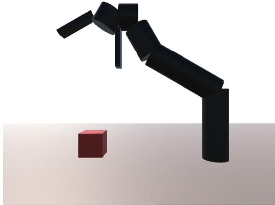
FIGURE 6.2: The starting position of an experiment where the cube position and joint angles are kept constant at the start of each episode. Intermediate rewards are used to guide the agent to interesting state spaces.
