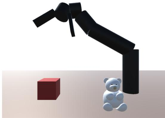
FIGURE 6.15: An example of introducing clutter into the scene in the form of a bear. We test the agent to see how well it generalises when adding in clutter without any further training.
