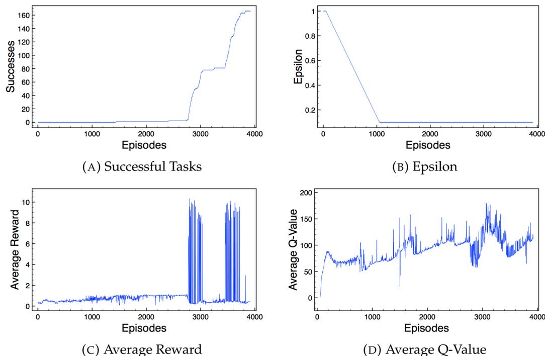
FIGURE 6.18: The results of running  $\epsilon$ -greedy with a simple fully connected network with no visual input.
