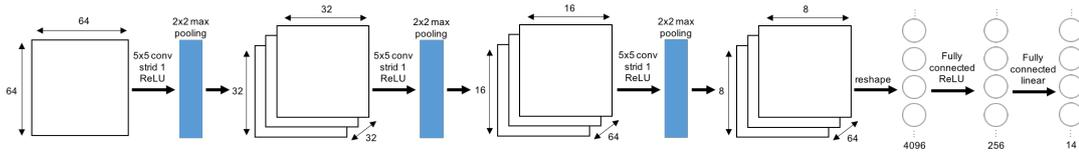
FIGURE 4.4: Our convolutional neural network architecture consisting of 3 convolutional layers and 2 fully connected layers. The network accepts  $64 \times 64$  resolution grayscale images and outputs motor actions.
