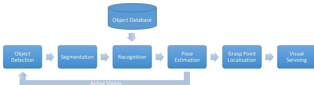
FIGURE 1.1: Traditional active vision pipeline for object manipulation.
