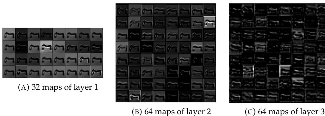
FIGURE 6.12: The activations in the feature maps of the trained network during the agent's attempt to pick up the cube from different starting positions and joint angles. Activations have gotten stronger since being trained to generalise.
