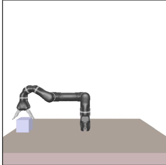
FIGURE 5.4: The starting position of our first successful experiment that picks up the cube. Joint angles are set like this so that the probability to pick up the cube is higher than in the previous experiment.
