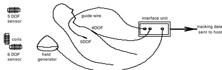
**Fig 1:** The basic configuration of using Aurora electromagnetic tracking systems in a clinical setting for removing global patient motion and recovering respiratory pattern.
