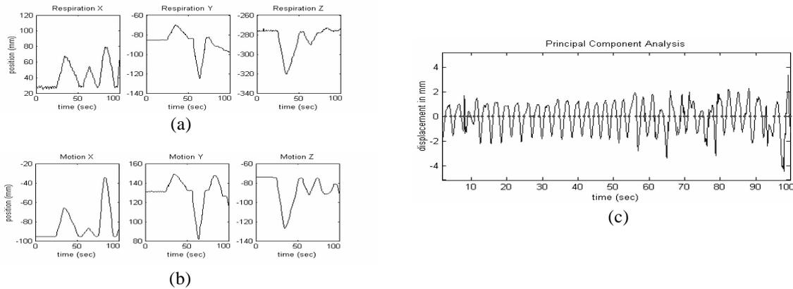
**Fig 2:** Example position traces sampled by the EM tracker and the extracted respiratory motion pattern. (a) x, y, z positional component of the data received from the EM tracker attached on the chest of one of the subjects, (b) x, y, z positional component of the data received from the EM tracker attached on the couch, (c) The recovered respiratory component.
