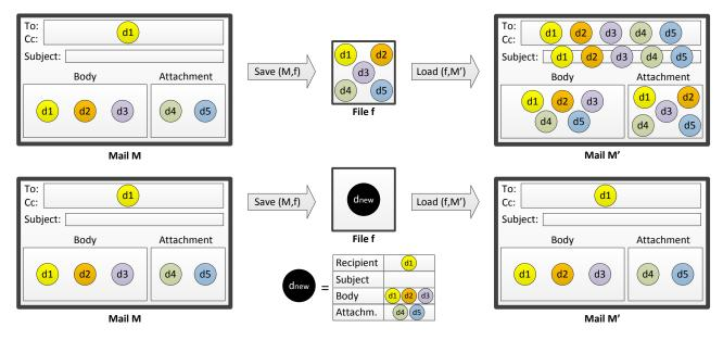
Fig. 1. Result of tracking the flow of data while saving a mail to a file and reopening it with (above) and without (below) the use of structured taint marks.
