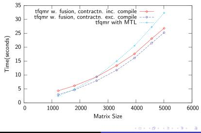
256 iterations of BiConjugate Gradient Solver on Rays.
