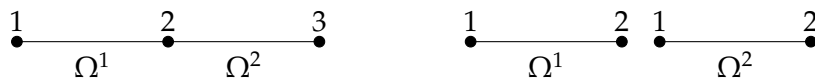
Figure 2.7: Left : A 1D domain decomposed into two elements ( \Omega^i ). Right : Local node numbering of individual elements.
