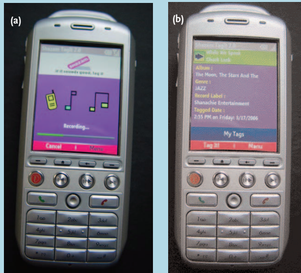
Shazam interface: (a) recording a 10-second audio sample; (b) displaying the query results.
