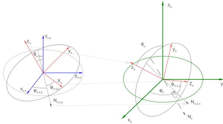
**Fig. 11** Euler angles between  $n$  and  $n-1$  cross section frame;  $n$ -th cross section frame shown with the global frame
