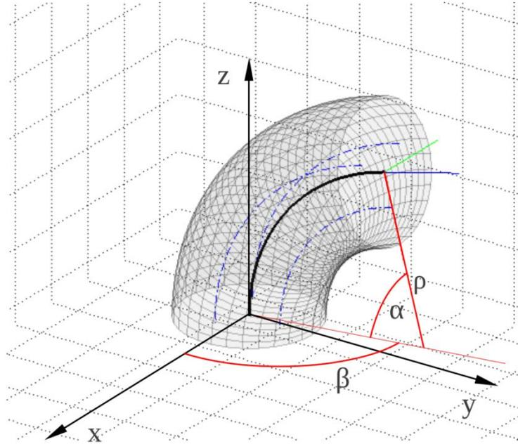
**Fig. 5** Module bending with no external forces applied
