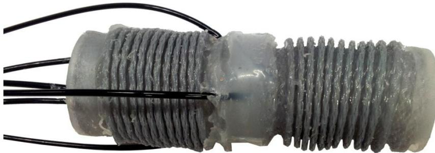
**Fig. 3** Photograph of a two segment arm manufactured by partner from the Stiff-Flop project
