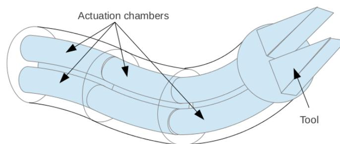
**Fig. 1** Visualization of the Stiff-Flop manipulator
