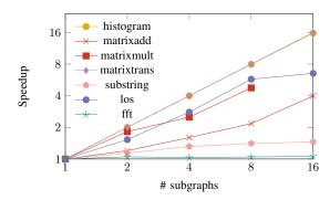
Fig. 8: Speedup, compared to original Dynamatic, as more subgraphs in the CFG are parallelised.
