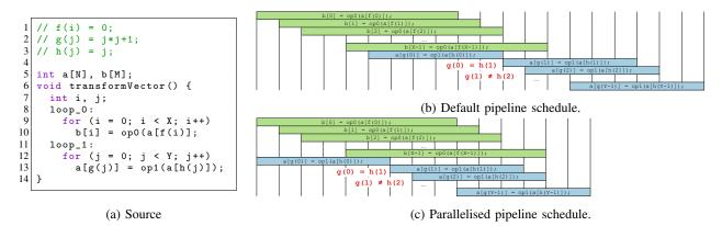
Fig. 2: Motivating example. Assume no dependence between two loops. The dynamically scheduled hardware from the original Dynamatic [1] computes in the schedule in (b). Our work achieves an optimised schedule in (c).
