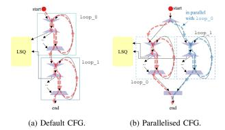
Fig. 1: Transformation of control flow graph (CFG) for the example in Fig. 2. Our toolflow enables multiple BBs to start simultaneously to achieve the schedule in Fig. 2c.
