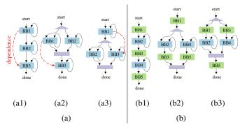
Fig. 4: A CFG may be parallelised differently, depending on (a) parallelising in top-to-bottom/bottom-to-top order, and (b) grouping BBs with the loop before/after. The dashed arrows represent memory dependence.
