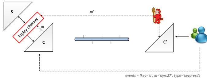
**Figure 3:** Architecture of RIPLEY: user events are delivered to both the JavaScript client-side component  $C'$  and its server-side replica  $C$ . RPCs arriving from both to the server component  $S$   $m$  and  $m'$  are compared by the RIPLEY checker.
