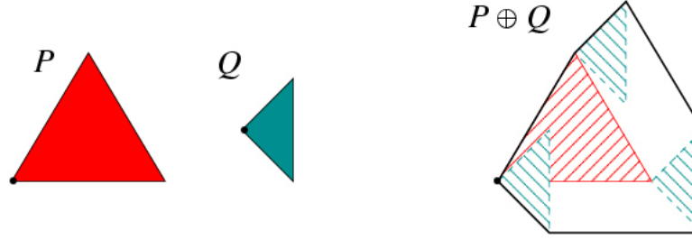
Figure 2.1: The figure shows the Minkowski addition of two convex 2D-simplices (triangles), following the definition [7]. The result is by a convex shape, as a result of the minkowski sum properties. The bullet marks the origin (0,0) for each shape.
