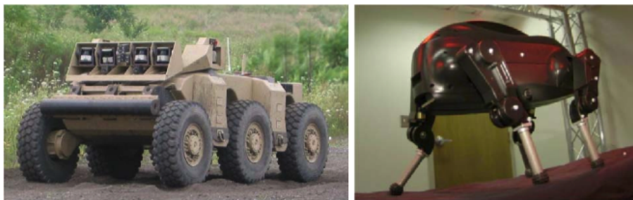
Figure 1.4: From left to right: 1. Autonomous ground vehicle Crusher, built by the National Robotics Engineering Center(NREC). 2. Quadruped robot LittleDog, built by Boston Dynamics. Taken from Ratliff et al. (2009b)
