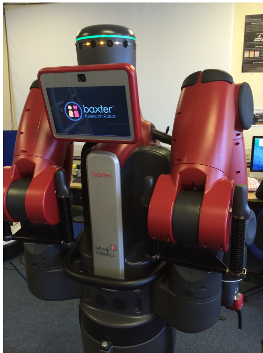
Figure 1.1: A photo of the Baxter robot. This robot was taught to learn to sweep with a dustpan and brush from a single demonstration, as an example of apprenticeship learning.
