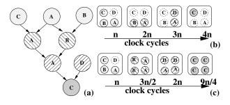
Figure 1. Motivating example. (a) Data flow graph. (b) Static implementation, showing which function units are inactive (with dotted boundaries) from time=0 to 4n cycles. (c) Dynamic implementation.
