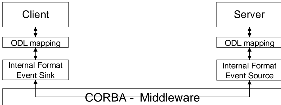
Figure H.1: The Event System Architecture
