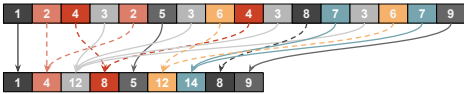
Fig. 3. Local to global mapping for 2x2 quadrilateral mesh, P=1 , applied to a vector in local coefficient space.
