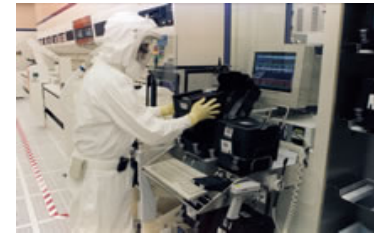
Intel technicians monitor wafers in an automated wet etch tool. The process cleans the wafers of any excess process chemicals or contamination.
