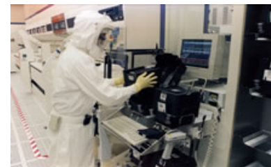
Intel technicians monitor wafers in an automated wet etch tool. The process cleans the wafers of any excess process chemicals or contamination.
