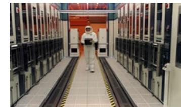
Checking wafers processing in a vertical diffusion furnace
