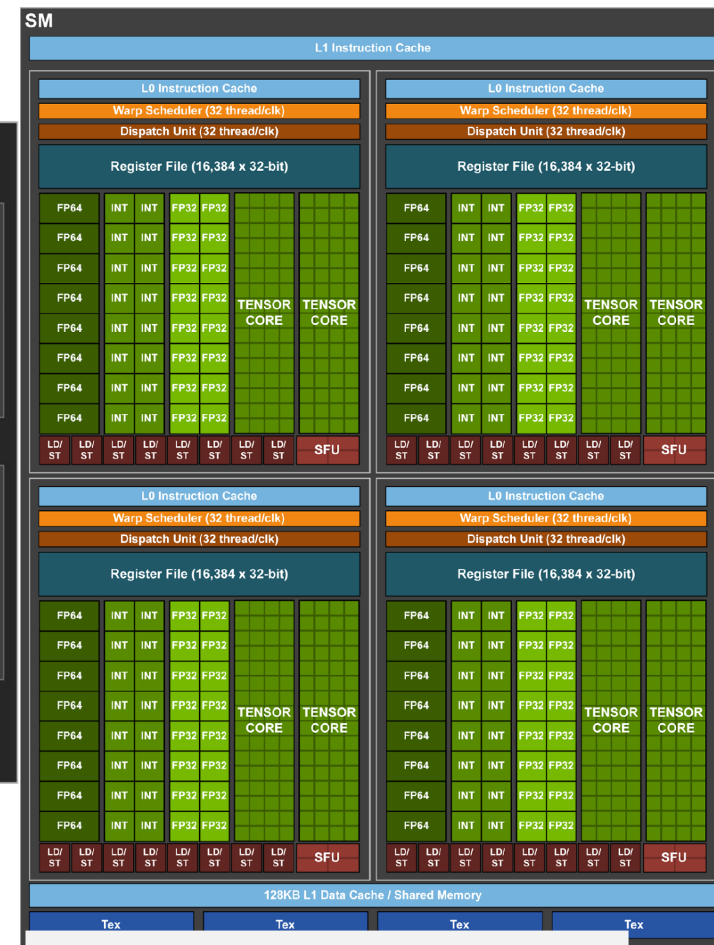
GV100's SM includes 8 tensor cores
