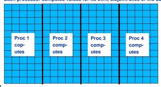
Each processor computes values for its own, disjoint slice of the data
