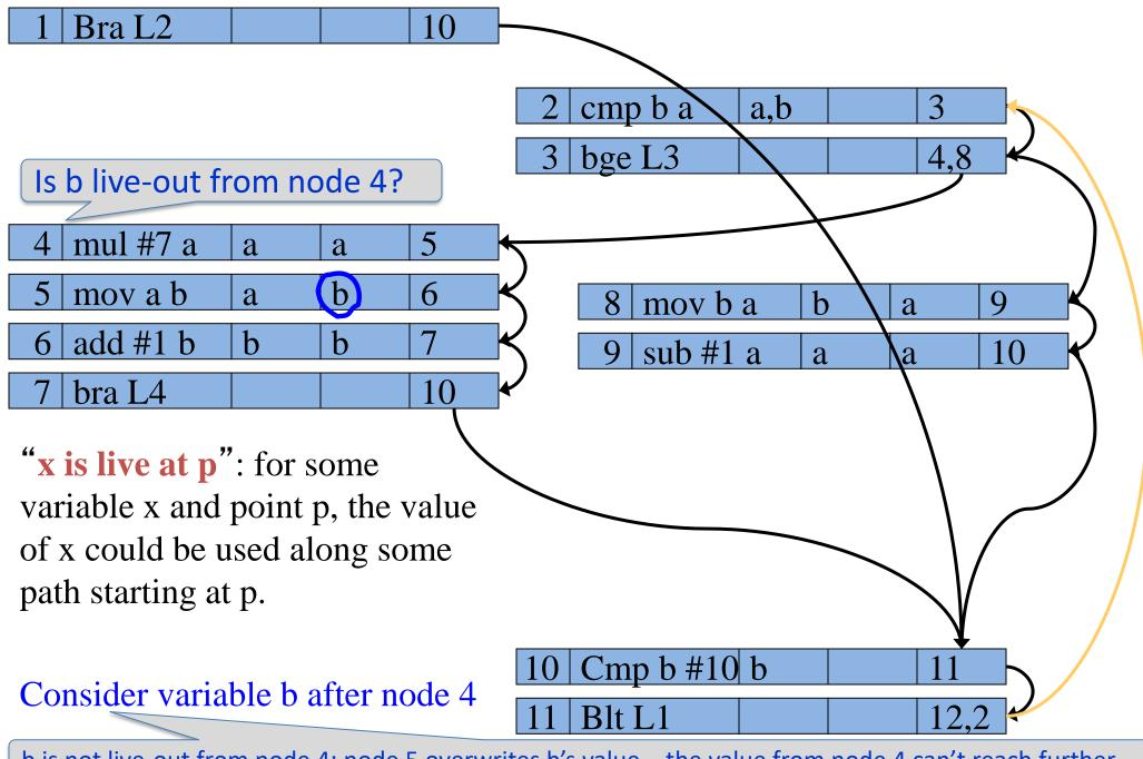
b is not live-out from node 4: node 5 overwrites b's value – the value from node 4 can't reach further
