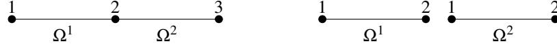
Figure 1: Left : A 1D domain decomposed into two elements ( \Omega^i ). Right : Local node numbering of individual elements.
