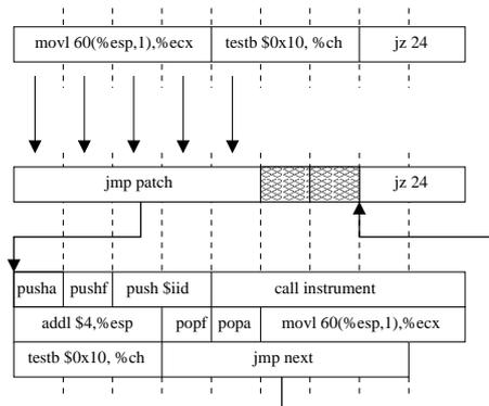
Fig. 1: *Illustrating the process of placing a code splice. In the new sequence two bytes are now redundant, as they are no longer in the flow of control. The two overwritten instructions are relocated to the patch.*
