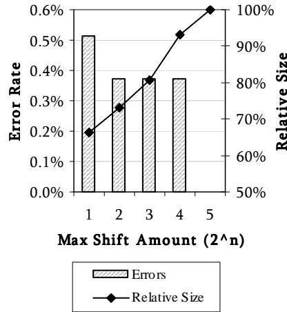
Fig. 5: Graph showing the variation of error rate and hardware size with maximum shift amount for the “swim” benchmark.
