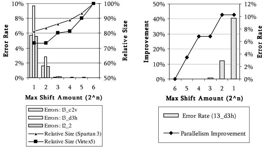
(b) Graph showing variation of error rate with maximum shift amount, for three datasets, overlaid with relative hardware size on two test systems
