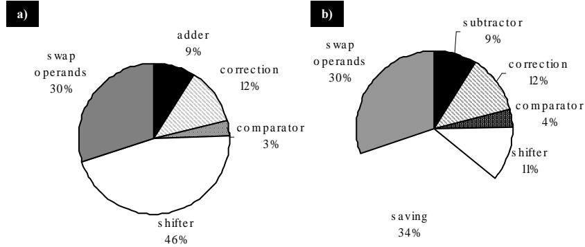
Fig. 2: Charts showing resource distribution, given as Altera Stratix II ALUTs, between functional areas on a floating point adder from the RPL library (a) and the savings made by our optimisation (b). The components are as follows:
