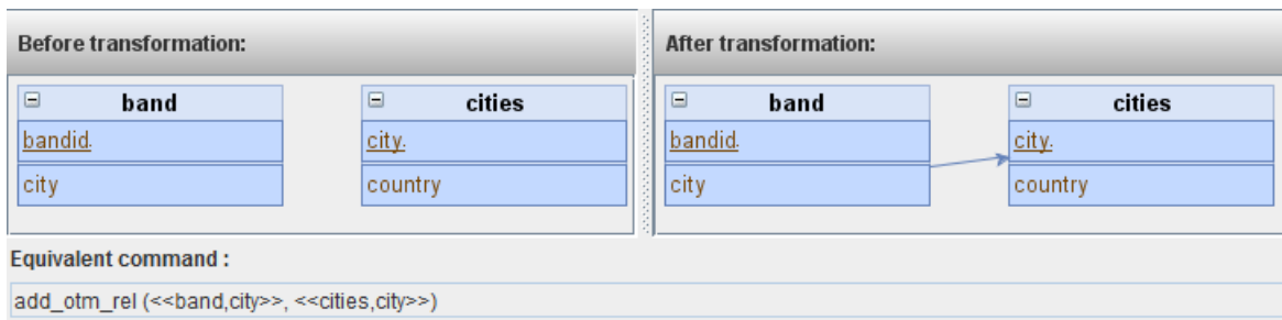
Figure 5.19: User interface for the addition of foreign key transformation.
