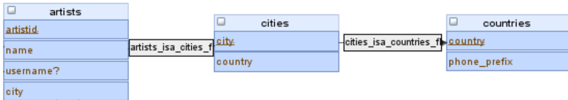
Figure 5.3: Schema in 3NF after the application of the normalisation pattern.
