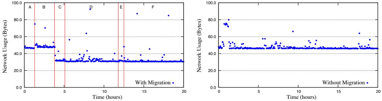
Figure 10. Network usage of a pair of queries, one with a migration (left) and one without (right)
