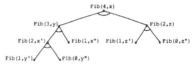
Here Fib(u,x) means the u-th Fibonacci number is x. Executing the same definition bottom-up generates the sequence of assertions
