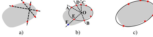
Fig. 3: Object detection: a) Sampled lines with edge points; b) Fitting of initial ellipse centred at  $O$ . Hypothesis tested using new edge points halfway between existing adjacent points. c) Revised hypothesis tested until hypothesis passes test.
