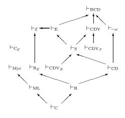
There is an arrow in this picture from one turnstyle to another if the system at the end of the arrow is an extension of the system at the start: if  $B \vdash M:\sigma$  holds in the system at the start of the arrow, then  $B \vdash M:\sigma$ holds in the system at the end; the latter M is sometimes obtained from the former one by bracket-abstraction. To summarize the general differences and similarities between the systems, we emphasize the following:
