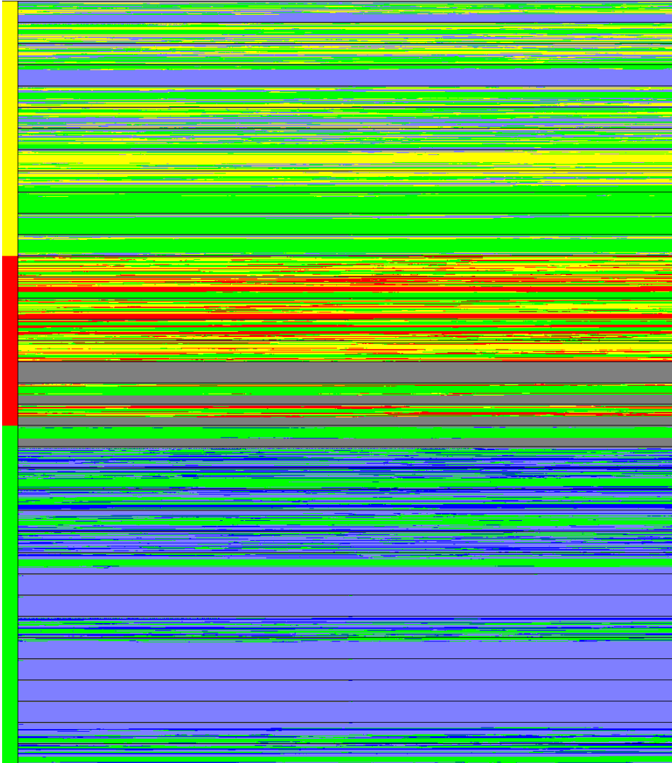
Figure 5.8.: Default ext3fs allocator bitmap for the read performance QoS attribute.
