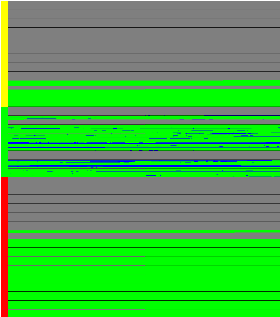
Figure A.4.: QoS-aware datablock allocator bitmap for the reliability QoS attribute on a reduced population filesystem.
