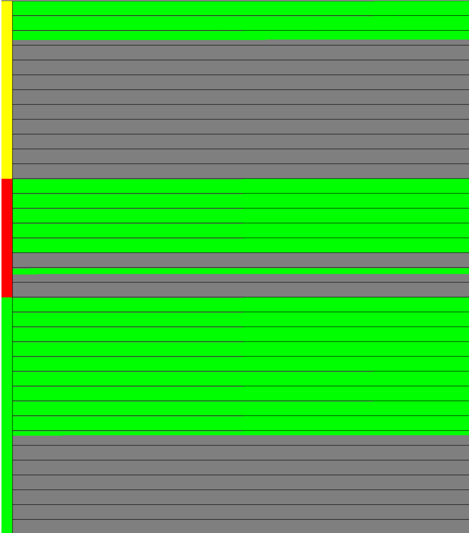
Figure A.3.: QoS-aware datablock inode bitmap for the write performance QoS attribute when using a reduced filesystem population.
