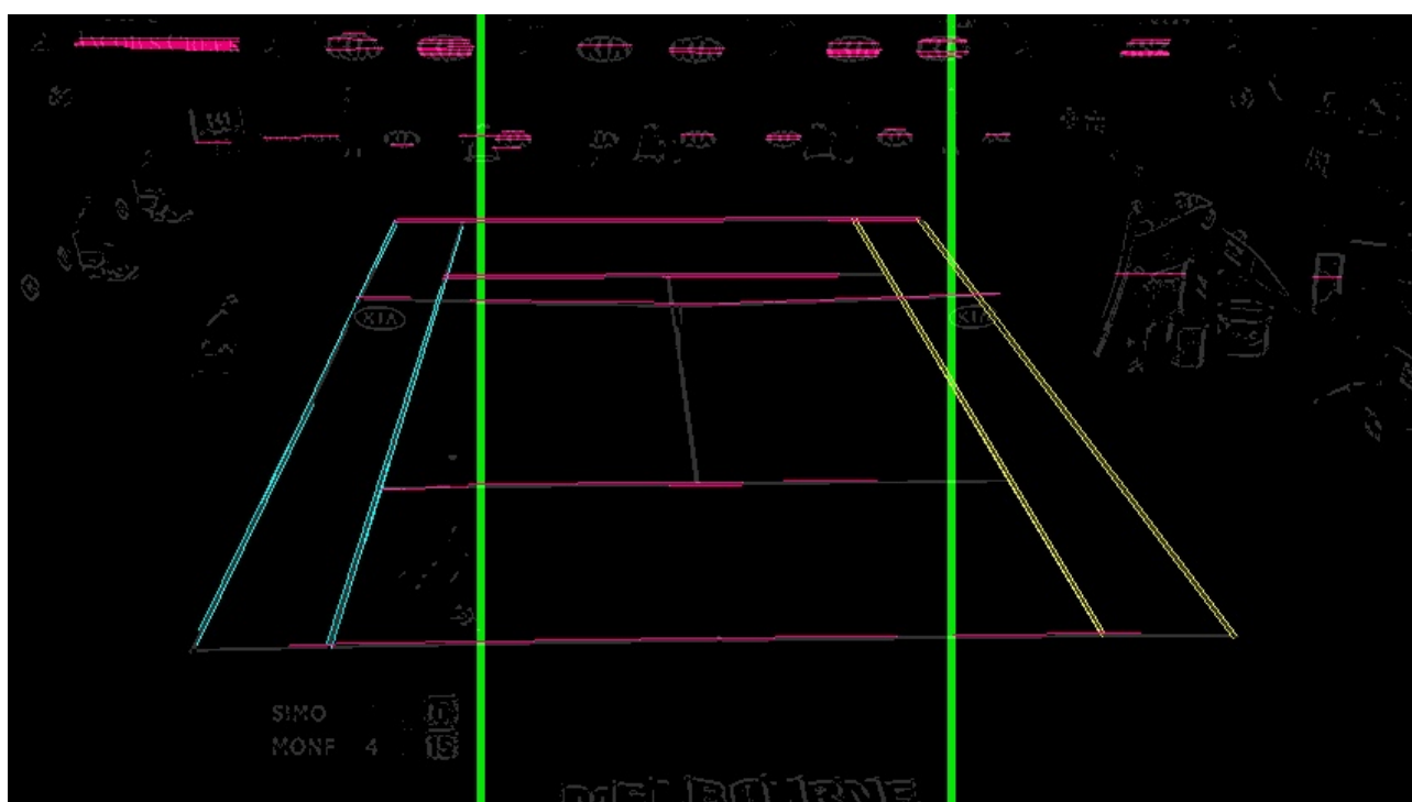
Figure B.2: Image resulting from lines extraction and classification into horizontal (magenta), left-vertical (blue) and right-vertical (yellow) lines.
