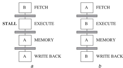
**Fig. 3** IMT and BMT multi-threading modes supported by CUSTARD
