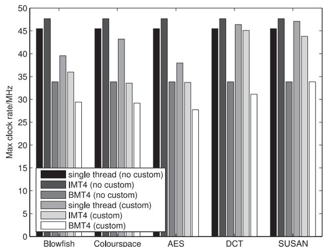
**Fig. 10** Maximum clock frequency for CUSTARD configurations as reported by Xilinx timing analyser
