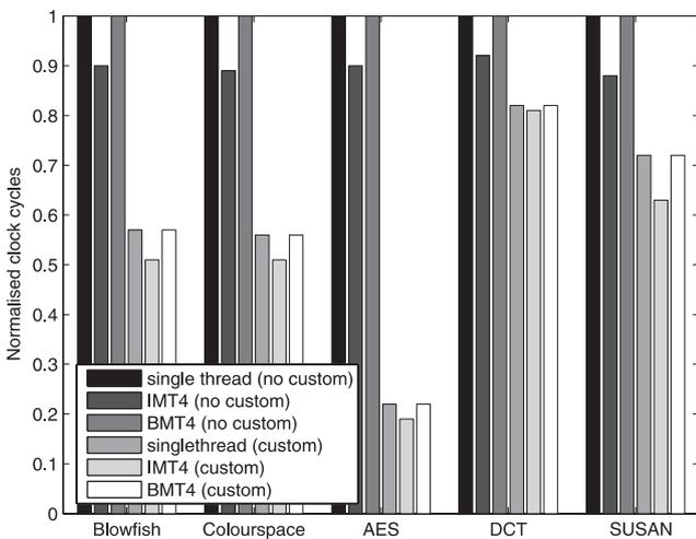
**Fig. 8** Normalised number of execution cycles required for six CUSTARD configurations running five benchmarks
