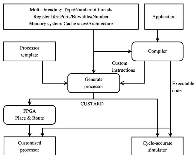
**Fig. 1** Toolflow for our processor customised for a particular application
