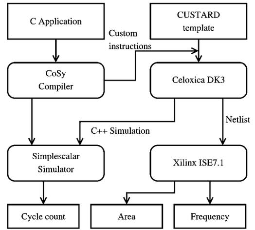
**Fig. 6** Implementation of our complete system, showing the source of each metric used to evaluate our processor designs
