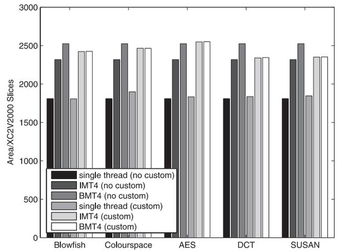
**Fig. 9** Required area in terms of XC2V2000 slices from a total of 21 504 for CUSTARD configurations
