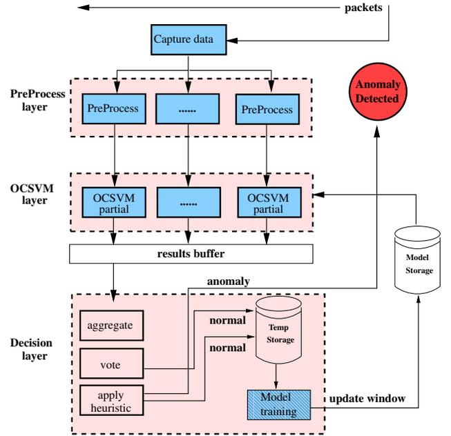
Fig. 3: DeADA architecture. Each blue box represents a computation node, at the various level. The *OCSVM layer* and *Decision layer* are the implementation of *USAE*. Note the *Model Training* node is stripped as this phase can be done via the architecture, or as an offline and separate process.
