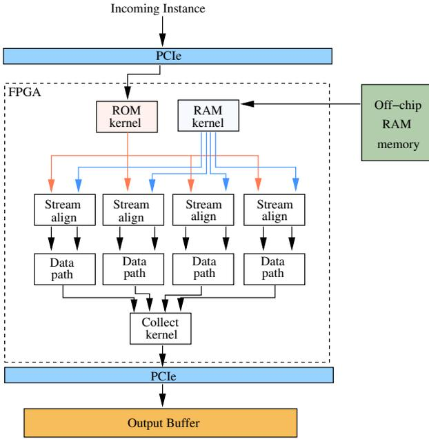
Fig. 4: FPGA architecture for OCSVM with USAE.
