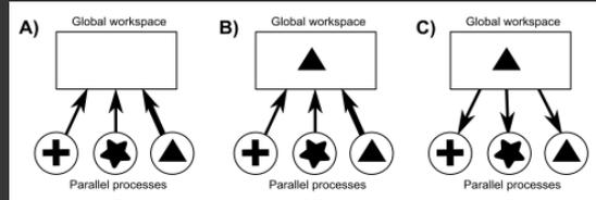
FIGURE 1. Generic operation of the global workspace architecture. A) Three parallel processes compete to place their information in the global workspace; B) The process on the right wins and its information is copied into the global workspace; C) Information in the global workspace is broadcast back to the parallel processes and the cycle of competition and broadcast begins again.
