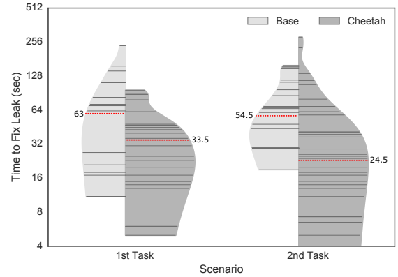
Figure 9: Violin plot representing the distribution of the times to fix leaks across all participants, by task and tool used during the task. Each horizontal line represents data leaks fixed in the task. The length of a line represents the number of leaks fixed in that time. Dashed lines are medians.
