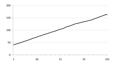
Figure 12: Memory footprint in MB as a function of the number of replicas.
