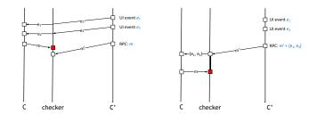
Figure 5: Eager (a) and lazy (b) event transfer. Events  $e_1$  and  $e_2$  arrive one after another. In **a**, they are sent over to the server right away. In **b**, they are queued-up and sent with the next RPC. While the overall completion time is later in the lazy case (as shown by a red filled square), one network message vs. three messages is used.
