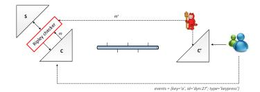
Figure 3: Architecture of RIPLEY: user events are delivered to both the JavaScript client-side component C' and its server-side replica C. RPCs arriving from both to the server component S m and m' are compared by the RIPLEY checker.
