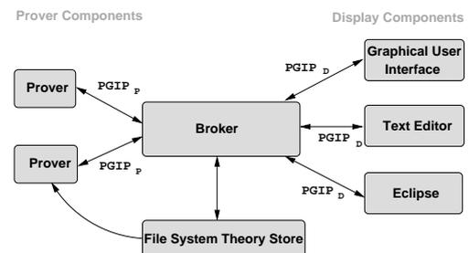
The syntax of *PGIP* messages is defined by an XML schema written in RELAX NG. Every message is wrapped in a `<pgip>` packet which uniquely identifies its origin and contains a sequence number and possibly a referent identifier and sequence number.
