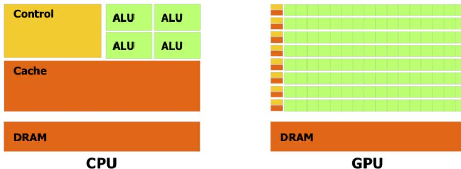
Figure 3.2: Processor Surface used for transistors: CPU / GPU [Credits: *nvidia*]
