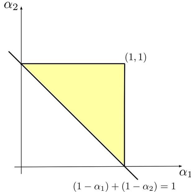
Figure 4.2: Support of two failed plants,  $B = 1$
