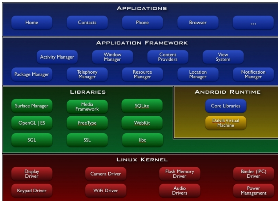
Figure 2.3: The Android Architecture [Goo11]
